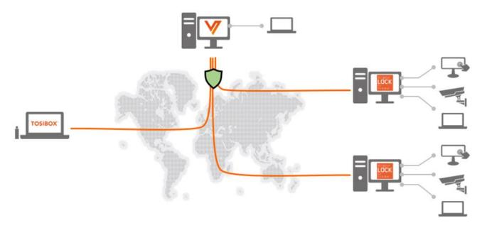
Figure 3: Connectivity from TOSIBOX® Key Client to devices behind TOSIBOX® Lock for Container via TOSIBOX® Virtual Central Lock
