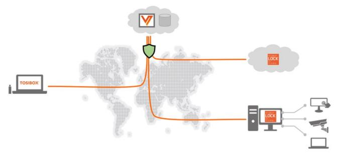
Figure 4: Connectivity from TOS/BOX® Key Client to cloud with TOS/BOX® Lock for Container via TOS/BOX® Virtual Central Lock
